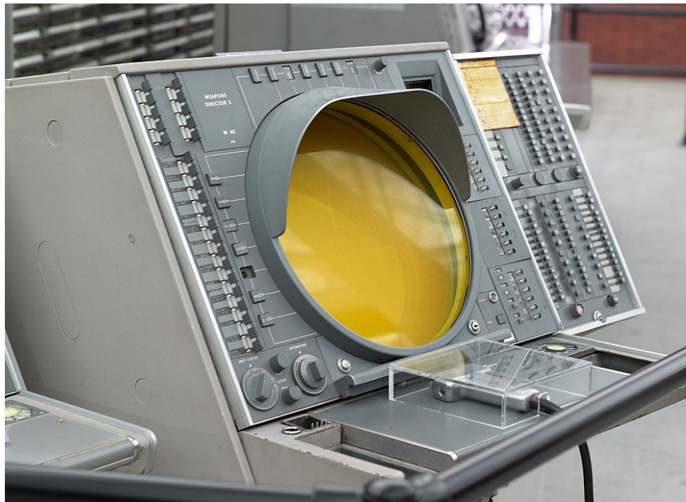
Semi-Automatic Ground Environment (SAGE) console (1958 –)
