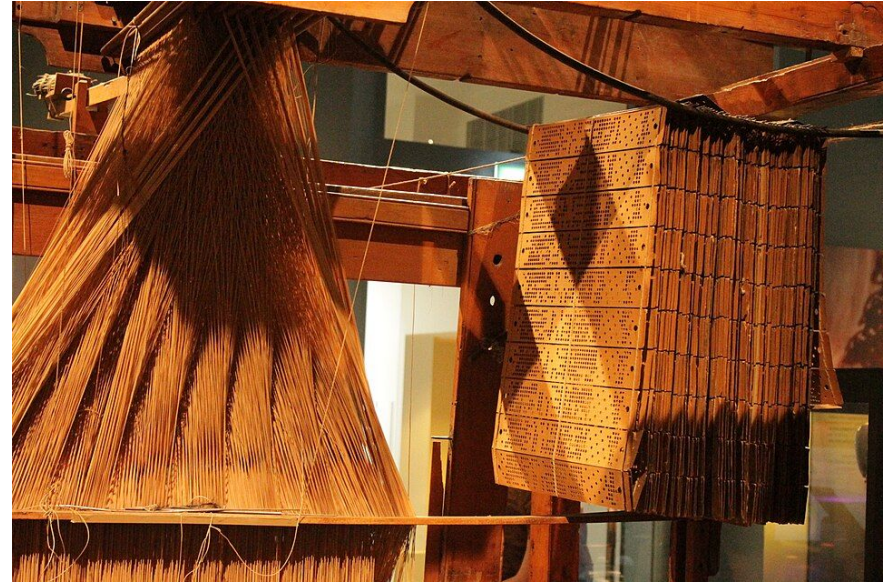
A Jacquard loom showing information punchcards (1800s) Photo © Wikipedia user Stephendickson CC BY-SA 4.0
