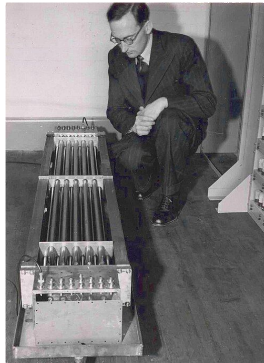
Maurice Wilkes inspecting the mercury delay line of the EDSAC (1949) in construction
